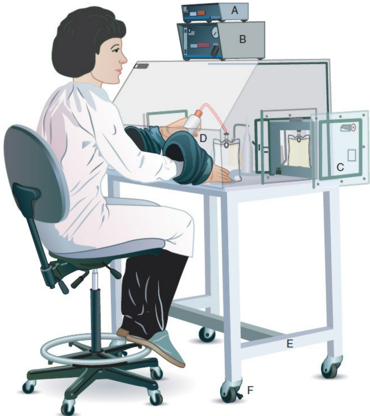
FIGURE 3-13 Glove box isolator.
