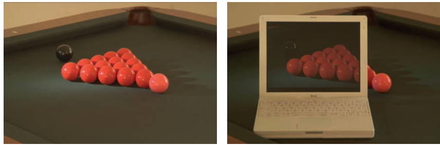
Figure 21.5. After tonemapping the image in Figure 21.4 and displaying it on a monitor, the monitor is placed in the scene approximately at the location where the image was taken. Dependent on the quality of the tone reproduction operator, the result should appear as if the monitor is transparent.
