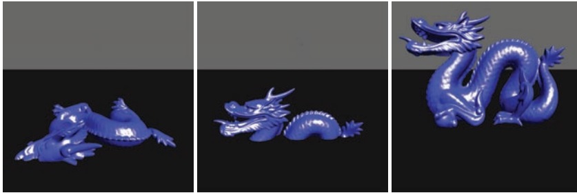
Figure 17.7. Images are described from left to right. The default local orientation of the dragon, lying on its side. After a -90 degree rotation about \vec{X} , the dragon is upright but still centered about the origin. Finally, after applying a translation of 1.0 in \vec{Y} , the dragon is ready for instancing.
