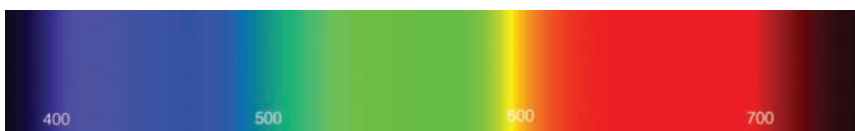
Figure 20.11. The visible spectrum. Wavelengths are in nanometers.
