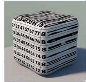
Figure 11.6. Using planar projection on a closed object will always result in a non-injective, one-to-many mapping, and extreme distortion near points where the projection direction is tangent to the surface.
