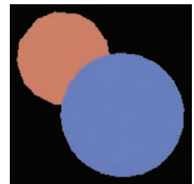
Figure 8.11. The result of drawing the same two spheres using the z-buffer .
