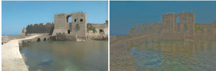
Figure 21.14. Bilateral filtering removes small details but preserves sharp gradients (left). The associated detail layer is shown on the right.
