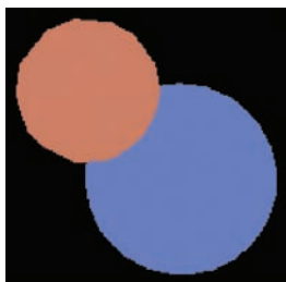
Figure 8.10. The result of drawing two spheres of identical size using the minimal pipeline. The sphere that appears smaller is farther away but is drawn last, so it incorrectly overwrites the nearer one.
