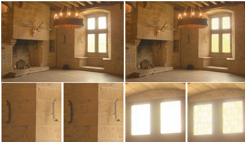
Figure 21.19. A global tone reproduction operator (left) and a local tone reproduction operator (right) (Reinhard, Stark, Shirley, & Ferwerda, 2002) of each image. The local operator shows more detail; for example, the metal badge on the right shows better contrast and the highlights are crisper.
