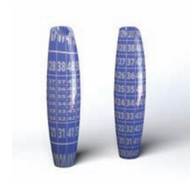
Figure 11.9. A far-from-spherical vase for which spherical projection produces a lot of distortion (left) and cylindrical projection produces a very good result on the outer surface.
