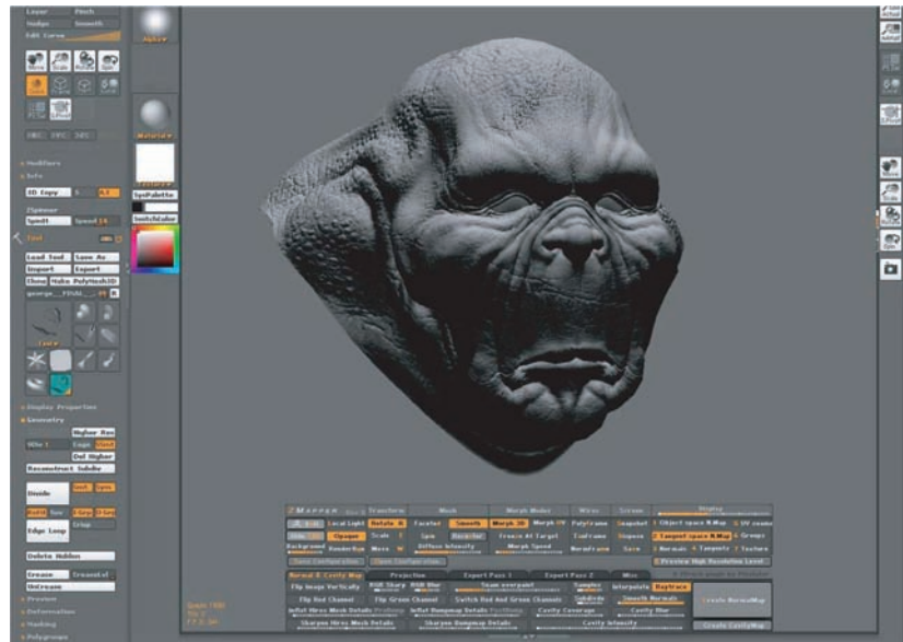
Figure 25.8. A visualization (in ZBrush) of the mesh from Figure 25.6, rendered with a normal map derived from the detailed mesh in Figure 25.7. The bottom of the figure shows the interface for ZBrush's "Zmapper" tool, which was used to derive the normal map. Image courtesy Keith Bruns.
