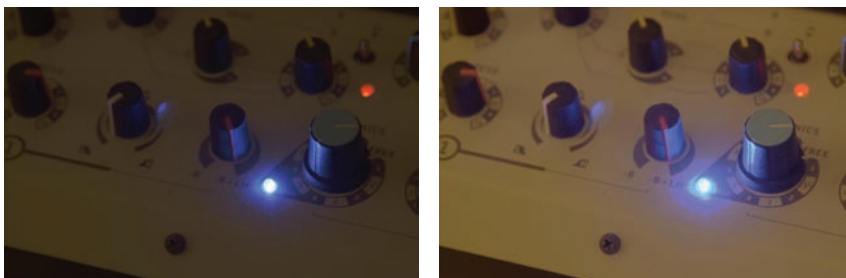
Figure 21.22. A linearly scaled image (left) and an image tonemapped using sigmoidal compression (right).
