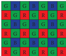
Figure 3.8. Most color digital cameras use a color-filter array similar to the Bayer mosaic shown here. Each pixel measures either red, green, or blue light.
