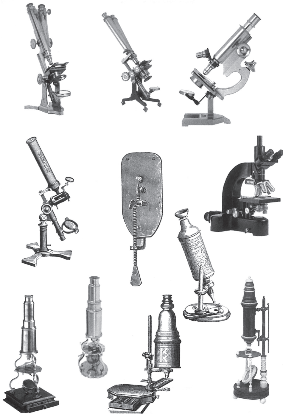
Figure 2-4. A simple Leeuwenhoek microscope (center), surrounded by examples of early compound light microscopes.
