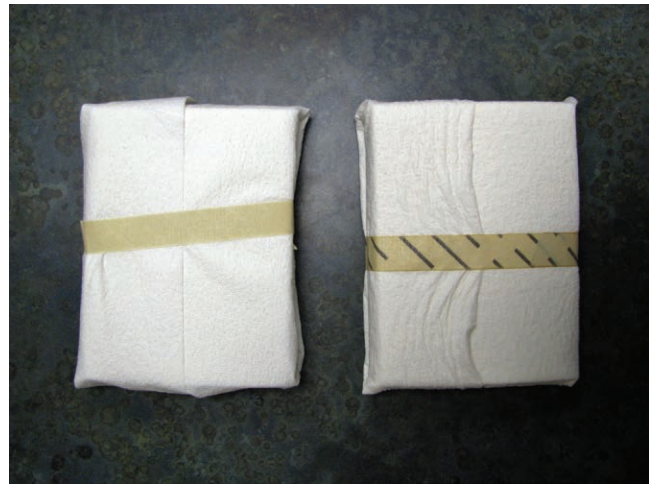
Figure 8-15. Autoclave tape. Left: Appearance of the tape before autoclaving. Right: Dark lines appear on the tape after autoclaving. The dark lines indicate that the proper temperature was achieved. (Courtesy of Dr. Robert Fader and Biomed Ed, Round Rock, TX.)
