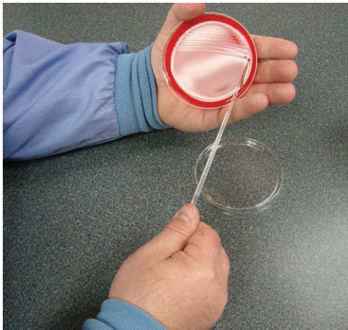
Figure 8-10. Laboratory professional demonstrating the proper method of inoculating the surface of an agar plate. The plate is held in the palm of one hand. The other hand is used to lightly drag the inoculating loop over the surface of the solid culture medium. The inoculating loop is held in much the same manner as a small camel-hair paint brush is held by an artist when applying paint to the surface of a canvas. This person would be wearing gloves if an actual specimen was being inoculated to the agar plate. (Additional information regarding the proper method of “streaking” can be found on thePoint .) (Courtesy of Dr. Robert Fader and Biomed Ed, Round Rock, TX.)
