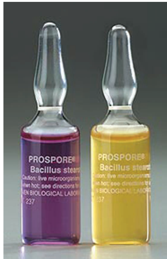
Figure 8-16. Biological indicator used to monitor the effectiveness of autoclaving. Sealed ampules containing bacterial spores suspended in a growth medium are placed within the load to be sterilized. Following sterilization, the ampules are incubated at 35°C. If the spores were killed, there will be no change in the color of the medium; it will remain purple. If the spores were not killed, germination will occur, and acid production by the bacteria will cause the pH indicator in the medium to change from purple to yellow. (Courtesy of Fisher Scientific.)
