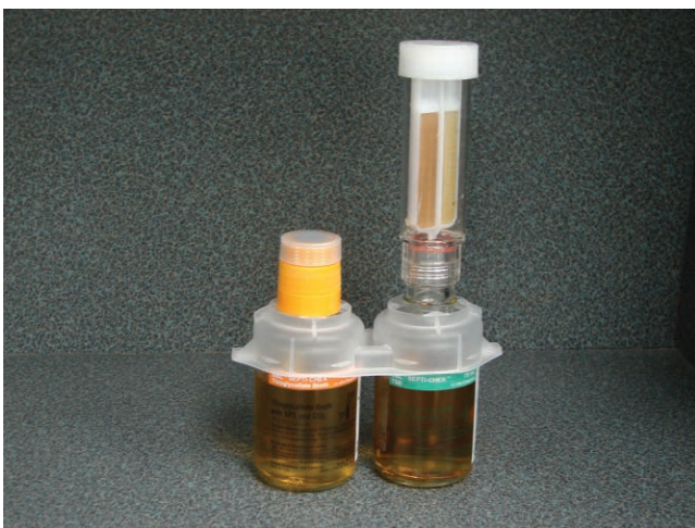
Figure 13-5. An example of a commercial blood culture system. The Septi-Chek blood culture system, manufactured by BD Biosciences, Franklin Lakes, NJ. The system consists of two bottles; an aerobic bottle and an anaerobic bottle. The aerobic bottle to the right is a biphasic system, consisting of a broth-containing vial with an attached agar-coated plastic paddle. (Courtesy of Dr. Robert Fader and Biomed Ed, Round Rock, TX.)
